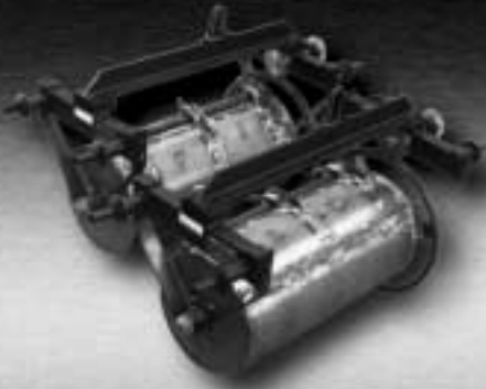
Two Model 2MMUSD 14"x30" gear driven round barrels. Cylinders are constructed of 12 ga. Monel with 1/8" perforations. A 96 tooth cylinder ring provides a 4.6:1 ratio. Upper superstructures are protection coated, mild steel. The barrels are tank supported with a Strap hangerarm arrangement.
