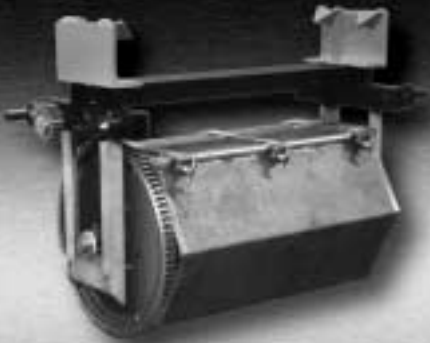
Model 2MS6SUSD 20"x36" gear driven phosphating barrel, constructed of T-316 stainless steel. The hexagon cylinder has 3/16" perforations. The barrel is tank supported with an Angle Iron hangerarm arrangement.
