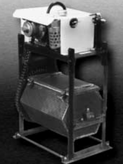
Model 2MSTBPOMC 12"x18" chain driven barrel is constructed of 12 ga. steel. The hex cylinder has 1/4" perforations. The variable speed overhead air motor delivers a cylinder speed of 2-5 RPM. The barrel has a Self Standing hangerarm arrangement.
