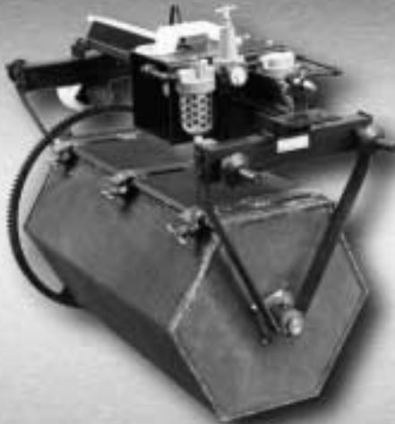
Model 2MS4HOMC 14"x30" black oxide processing barrel. The hex cylinder is constructed of 14 ga. T-304 stainless steel with 3/32" perforations. The overhead variable speed air motor delivers a cylinder speed of .92 to 2.8 RPM. The upper superstructure is constructed of protection coated mild steel. The barrel is tank supported with a Strap hangerarm arrangement.
